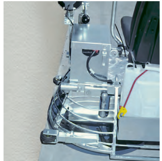
Equipped with device to float finishing wall edges
